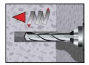
**1a**. Hammer (HD) or compressed air drilling (CD) Drill a hole into the base material to the size and embedment depth required by the selected anchor. Proceed with Step 2.
