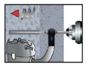
**1b.** Hollow drill bit system (HDB) Drill a hole into the base material to the size and embedment depth required by the selected anchor. This drilling system removes the dust and cleans the bore hole during drilling. Proceed with Step 3.
